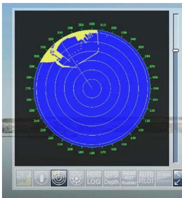
Figure 2: Small overlay display of basic radar. This can be shown on top of the 3D outside view screen.
